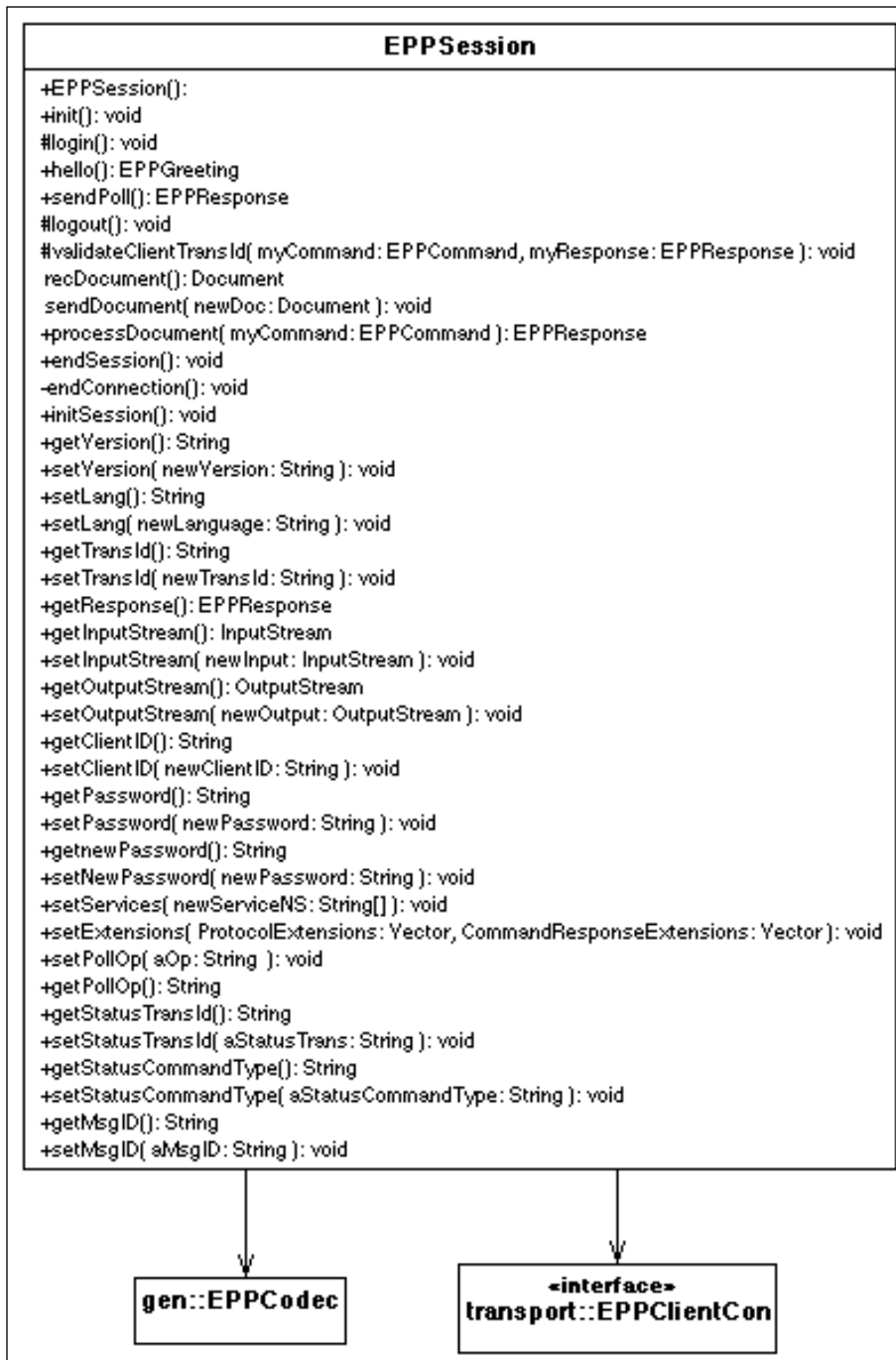
Figure 4 - EPPSession Class Diagram
